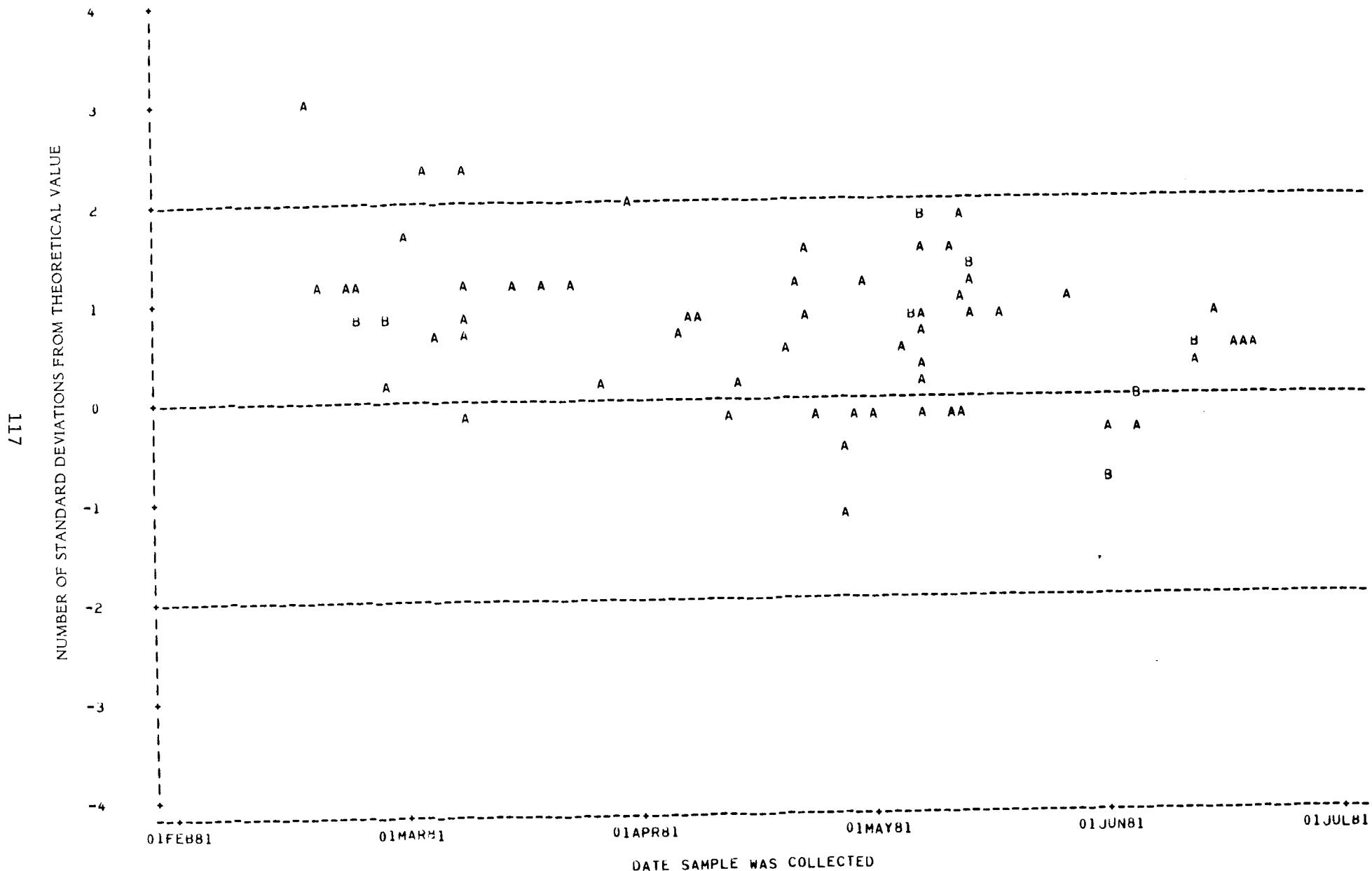
Figure A1.2.44.--Sulfate data for the Denver Laboratory.
